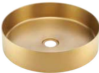
GB2.V400BL On Counter round basin, 304 stainless steel, 375mm - PVD brushed Brass - without overflow, without waste
