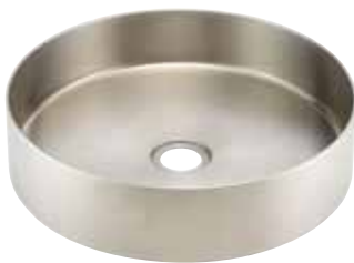
GB2.V400SS On Counter round basin, 304 stainless steel, 375mm - brushed stainless steel - without overflow, without waste
